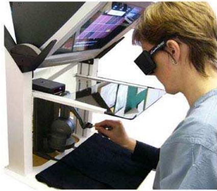
Figure 3. Spinal anaesthesia training system developed by DBMT [14]
